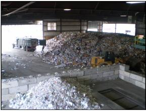
Recyclable materials are dropped off at the facility in a single-stream, meaning the materials do not have to be separated to be processed.
